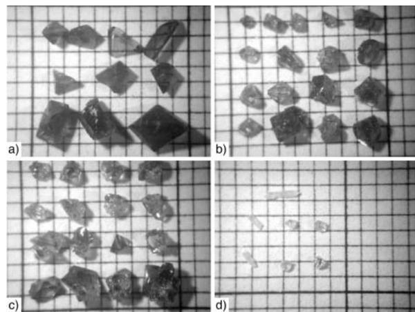
**FIGURE 2.** Photographs of experimental products produced with the  $\text{Na}_2\text{CO}_3\text{-MoO}_3$  flux alone. (a)  $\text{HoPO}_4$ , (b)  $\text{ErPO}_4$ , (c)  $\text{TmPO}_4$ , (d)  $\text{LuPO}_4$ . Grid unit = 1 mm.
