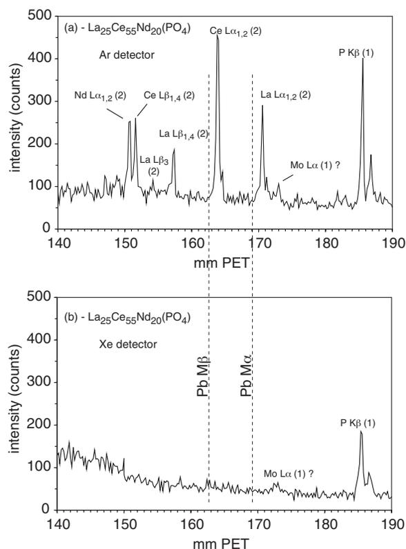
**FIGURE 6.** Enlargement of Figure 5f, showing a portion of the WD scan of  $(\text{La}_{0.25}\text{Ce}_{0.55}\text{Nd}_{0.20})\text{PO}_4$ , from 190–140 mm PET, for (a) the Ar detector and (b) the Xe detector. Approximate positions of the  $\text{PbM}\alpha$  and  $\text{PbM}\beta$  peaks are indicated by vertical lines labeled “ $\text{PbM}\alpha$ ” and “ $\text{PbM}\beta$ ”, respectively.
